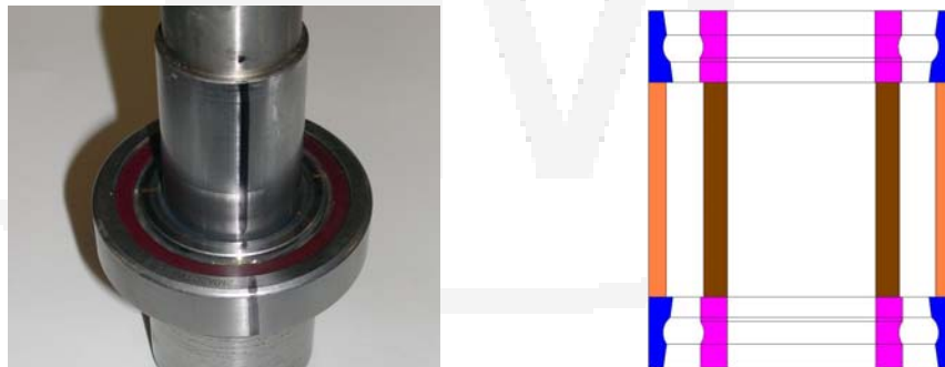
Figure 18 - Note the Axial Alignment Asterisk and the Bearing Orientation
