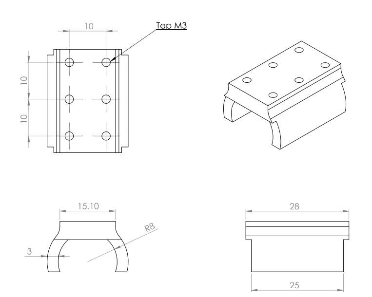
LME8UU linear bearing mount - 3d Printed in ABS Mass of printed part at 100% fill = 3.5g
